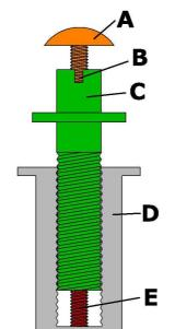
A: Top screw B: Slot for bridge height adjustment C: Bridge stud bolt D: Threaded insert E: Base screw
