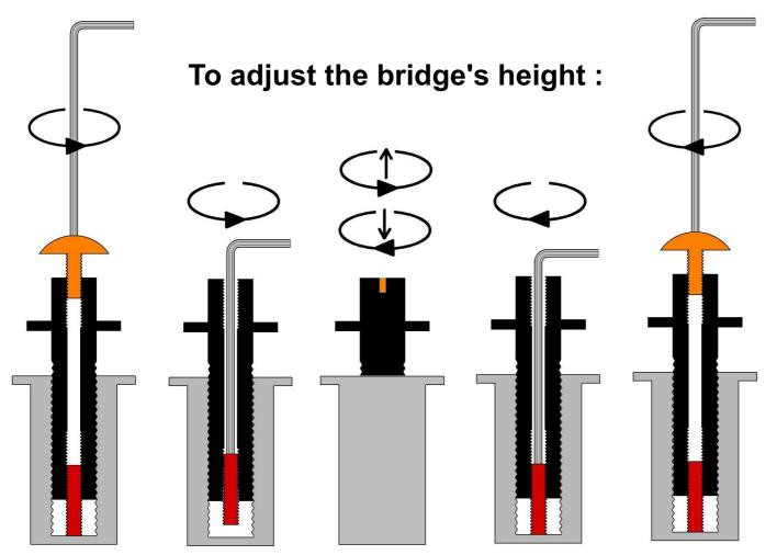
The "E" base screw's pourpouse is to firmly lock the "C" bridge Stud bolt in it position, while the "A" top screws pourpouse is to lock the bridge to the "C" bridge stud bolt.
